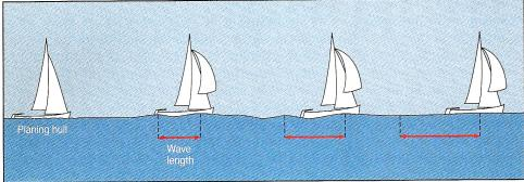
When a hull moves through the water, it produces waves that result in energy loss. The maximum speed of a conventional displacement hull (top) is a function of the longest wave it can make, which in turn is determined by hull length. No amount of sail can create enough power for it to climb over its own bow wave. On the other hand, the planing hull (bottom), like the racing dinghy and some multihulls, can carry enough sail to push it over its own bow wave and plane.
