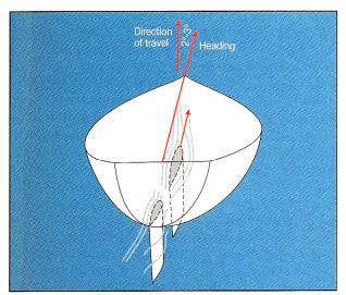
Since the keel and rudder must be presented to the water at a slight angle of attack (ideally 2° to 3°) in order to create maximum lift, the boat must be steered in one direction—its heading—to travel in a slightly different direction.
